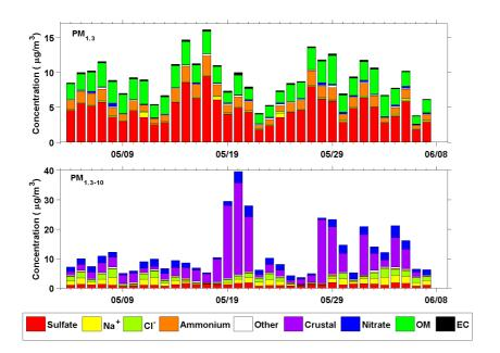
**Fig. 6.** Daily average of  $PM_{1.3}$  and  $PM_{1.3-10}$  during the study, based on filter measurements. OM was calculated as  $OC^*2.2$  according to Hildebrandt et al. (2010). Crustal concentration is calculated using iron as a surrogate according to Sciare et al. (2005). Other is the sum of  $PO_4^{3-}$  and  $K^+$ .
