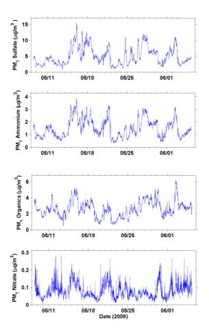
**Fig. 5.** Time series of  $PM_1$  aerosol composition measured by the Q-AMS. Different scales are used for each graph.
