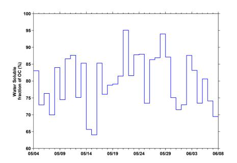
**Fig. 8.** Percentage of water soluble OC based on PM<sub>1</sub> filter measurements. On average 80% of OC was water soluble.
