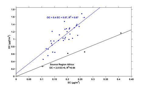
**Fig. 9.** OC versus EC as determined by  $PM_1$  filters. The slope of the OC versus EC line was 5.4 (blue points) for the study period with the exception of 19 to 21 May (source region Africa), when it was equal to 2.8 (black points).
