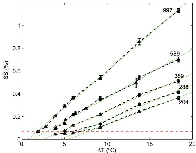
**Fig. 2.** Calibration of DMT-CCN instrument as a function of temperature gradient at different pressures (units: mbar). Green lines are best fits through the data. The red dashed-line represents 0.07% supersaturation (the lower operating limit of the CCN chamber; Roberts and Nenes, 2005).
