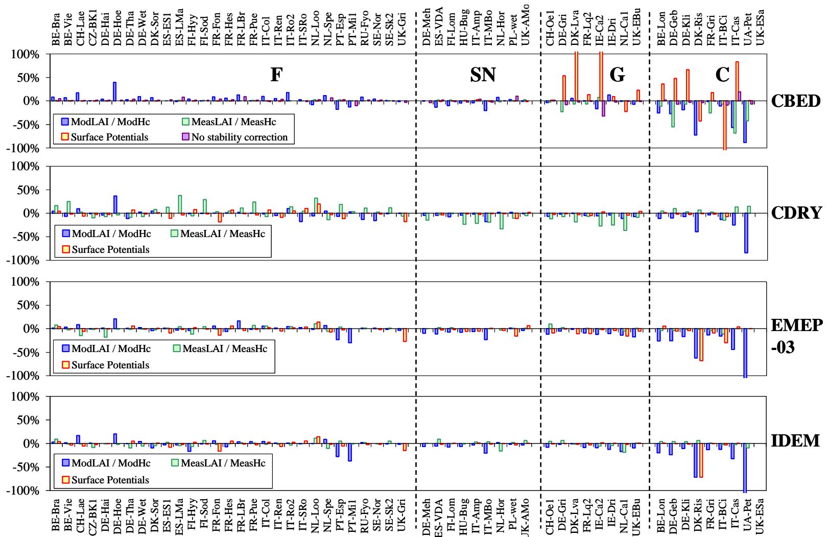
1 2 Figure A2. Sensitivity of modelled annual N_r dry deposition fluxes to the choice of input data for LAI, h_c (measured vs model default), to the 3 use of temperature and relative humidity at the surface ( d+z_0' ) rather than ambient, and to the non-implementation of stability corrections 4 (CBED only). The percentage differences are expressed relative to the model base runs as detailed in Table A2, with a negative number 5 indicating larger dry deposition (or smaller emission), and a positive number indicating smaller dry deposition (larger emission).
