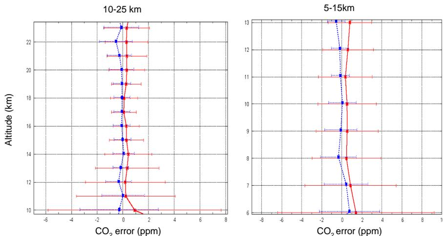
**Fig. 4a.** Results of synthetic retrievals of the CO<sub>2</sub> mixing ratio difference (in ppm) between the true profile and the retrieved profile (average over 20 occultations). Blue curve: all the uncertainties are considered as Gaussian random noise added to the “observations”; red curve: realistic temperature and species (N<sub>2</sub>O, O<sub>3</sub>, etc.) uncertainties are introduced in the atmospheric model; horizontal bars are one standard deviation.
