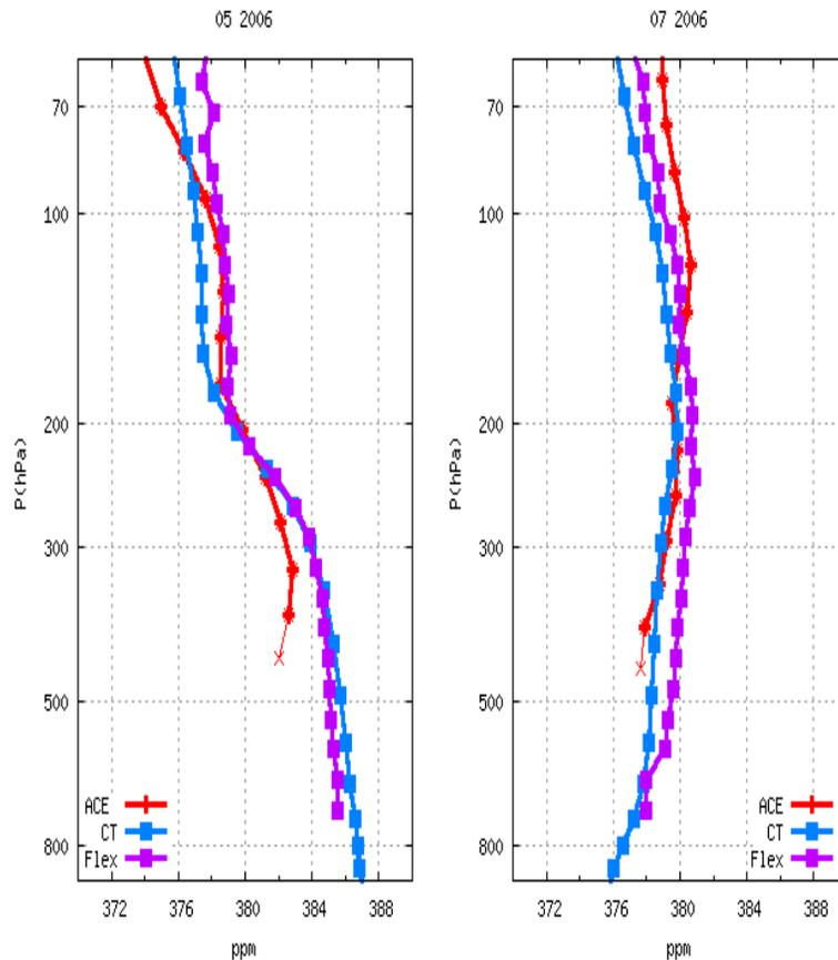
**Fig. 8.** CO<sub>2</sub> concentration (x-axis in ppm) evolution with pressure (y-axis in hPa) for May (left) and July (right) of 2006 for the 50° N–60° N latitude band. ACE-retrieved profile is in red, CT profile is in blue and Flexpart profile is in purple.
