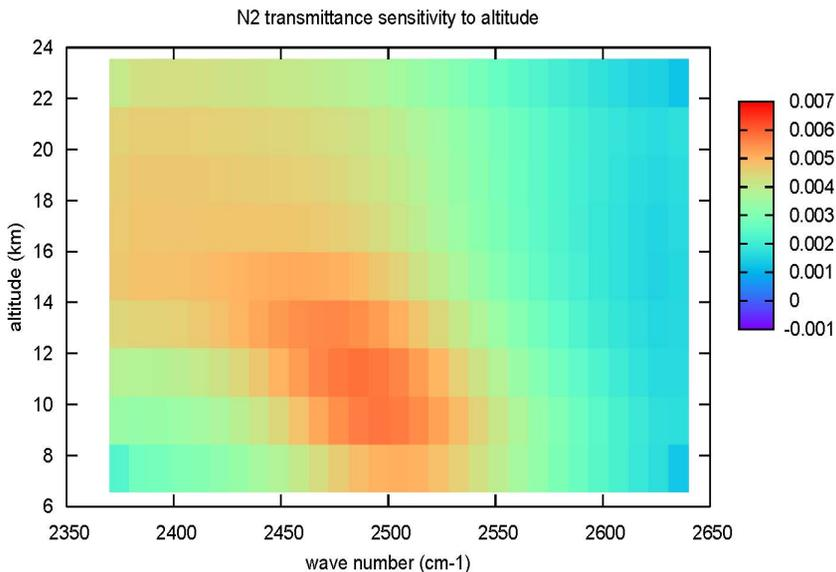
**Fig. 1.** Transmittance sensitivity to tangent height in the N<sub>2</sub> collision-induced absorption (2370–2640 cm<sup>-1</sup>) spectral range. The color bar values represent the transmission variation due to a 100 m tangent height change.
