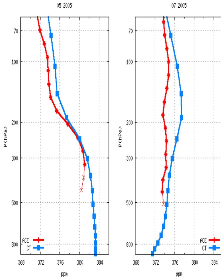
**Fig. 7.** CO<sub>2</sub> concentration (x-axis in ppm) evolution with pressure (y-axis in hPa) for May (left) and July (right) for 2005 for the 50° N–60° N latitude band. ACE-retrieved profile is in red and CT profile is in blue.
