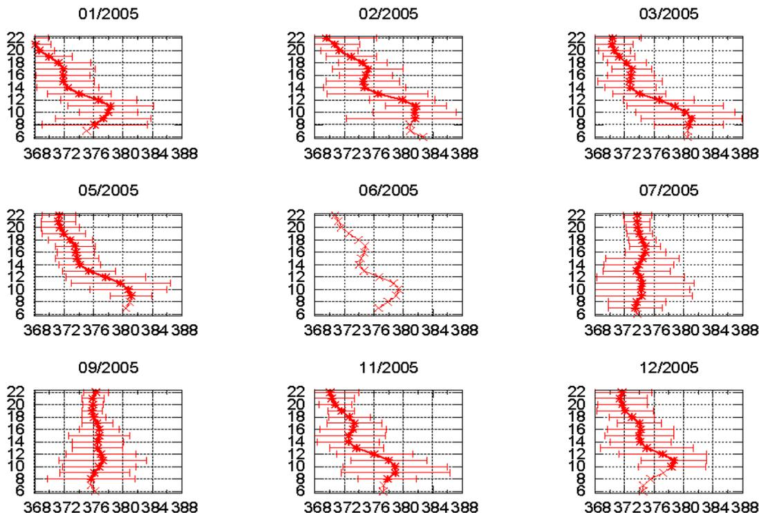
**Fig. A1.** Monthly mean CO<sub>2</sub> concentration (x-axis in ppm) evolution with altitude (y-axis in km) for nine months of 2005 for the 50° N–60° N latitude band.
