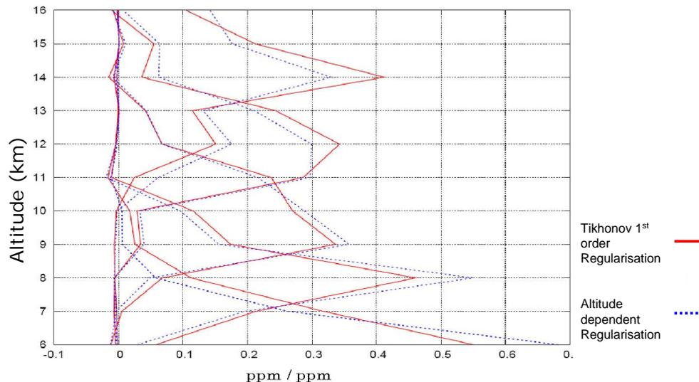
**Fig. 4b.** Averaging kernels for levels at 6, 8, 10, 12 and 14 km for one occultation. The red curve corresponds to a first order Tikhonov regularisation and the blue curve to an altitude dependent regularisation based on a Tikhonov first order operator.
