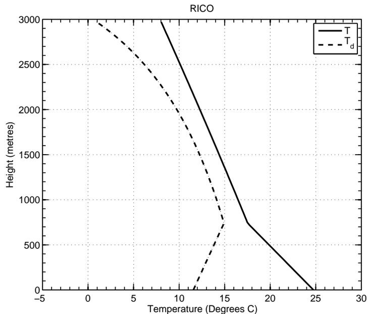
**Fig. 2.** Temperature (solid) and dew-point temperature (dashed) profiles in °C taken from the RICO model intercomparison, and used to initialise the models. The additional profiles, “RICO-2” and “RICO-5”, are obtained by cooling the RICO profile uniformly in height by 2 °C and 5 °C respectively under a fixed relative humidity.
