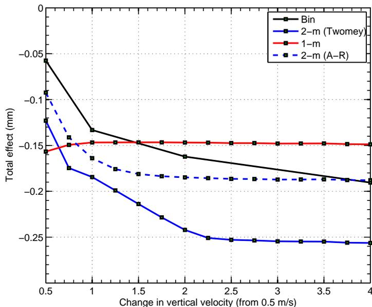
**Fig. 10.** Total effect on suppression of precipitation (in mm) from each scheme as a function of changes in  $w_1$  and CCN, under a fixed temperature ( $T=RICO$ ). Changes in  $w_1$  are considered from 0.5 m/s up to 4 m/s, and the change in CCN is from 50/cc to 100/cc.
