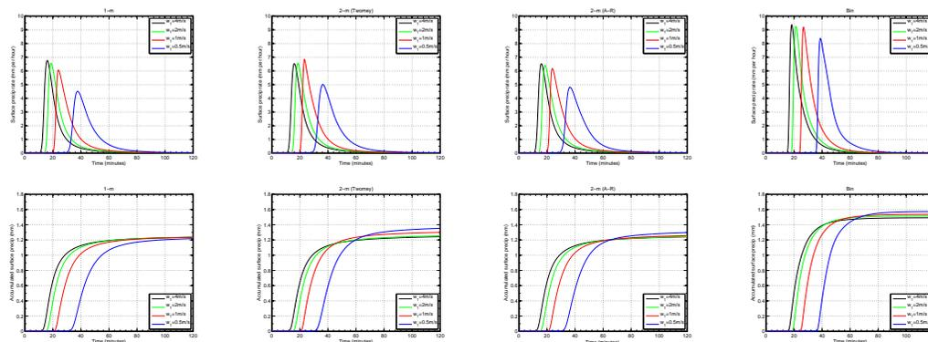
**Fig. 6.** Top row: timeseries of surface precipitation rates (mm/hr) from each scheme. From left to right: 1-m, 2-m Twomey, 2-m A-R, bin. Bottom row: the corresponding timeseries of accumulated surface precipitation (mm) from each scheme. Results are shown with  $CCN=100/cc$  and  $T=RICO$ , for four different values of  $w_1$ .
