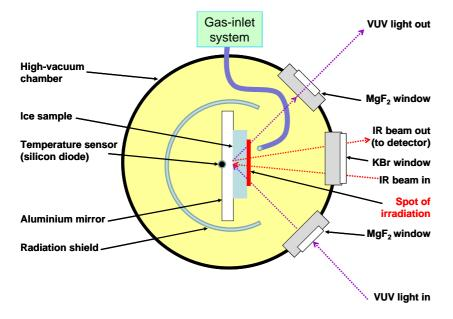
**Fig. 1.** Scheme of the laboratory setup illustrating the preparation of the ice film sample, its irradiation with VUV light be means of a hydrogen lamp and the measurement of IR spectra in the RAIRS mode.
