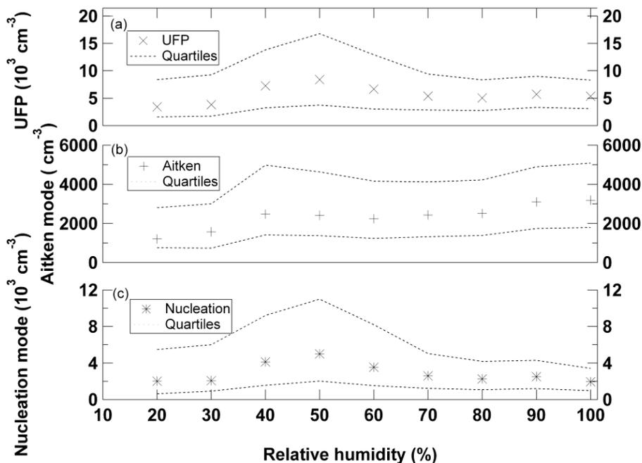
**Fig. 5.** Number concentrations of **(a)** ultrafine (UFP), **(b)** Aitken mode, and **(c)** nucleation mode particles and their variation as a function of relative humidity. The median number concentrations and the 1st and 3rd quartiles are presented.
