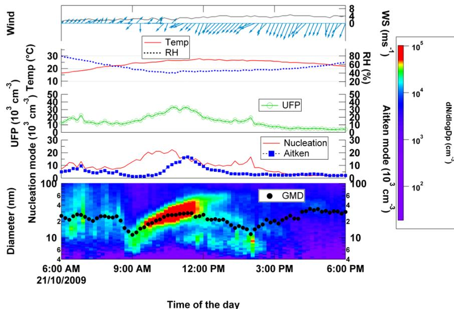
**Fig. 8.** The time series of nucleation events observed at QUT on 21 October 2009. From bottom to top, the parameters are: i) Geometric median diameter (GMD) and contour plot of size distribution; ii) Particle number concentration of nucleation and Aitken mode particles; iii) Particle number concentration of ultrafine particles (UFP); iv) Temperature and relative humidity; and v) wind direction and speed.
