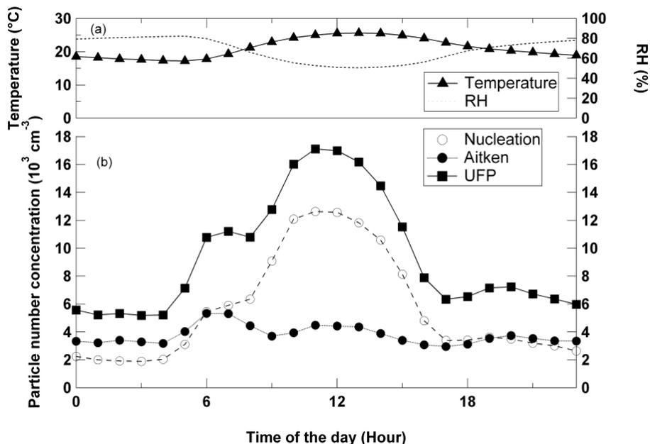
**Fig. 3.** Diurnal variation of (a) averaged temperature and RH and (b) averaged UFP, nucleation mode and Aitken mode particle concentrations.
