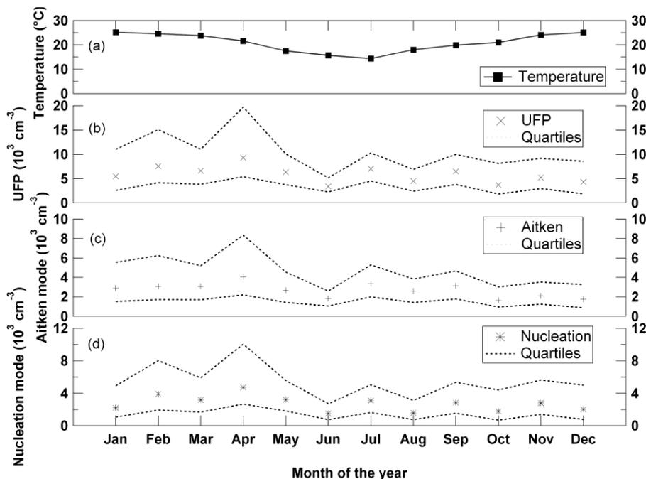
**Fig. 2.** Monthly variations of (a) mean temperature, (b) particle number concentration of ultra-fine (UFP), (c) Aitken mode, and (d) nucleation modes particles. The median number concentrations and 1st and 3rd quartiles are presented.
