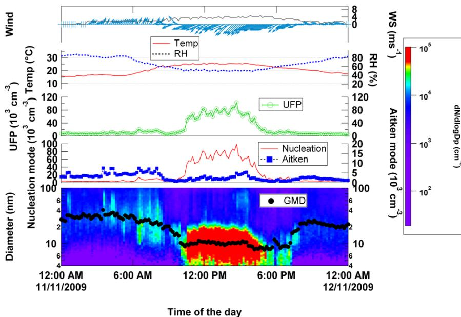
**Fig. 11.** The nucleation bursts measured on 11 November 2009. From bottom to top, the parameters are: i) Geometric median diameter (GMD); ii) Particle number concentration of nucleation and Aitken mode particles; iii) Particle number concentration of ultrafine particles (UFP); iv) Temperature and relative humidity; and v) wind direction and speed.
