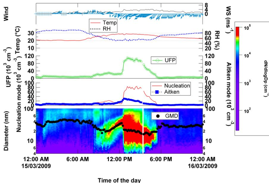
**Fig. 12.** Contour plot of particle size distribution observed on 15 March 2009. From bottom to top, the parameters are: i) Geometric median diameter (GMD) and contour plot of size distribution; ii) Particle number concentration of nucleation and Aitken mode particles; iii) Particle number concentration of ultrafine particles (UFP); iv) Temperature and relative humidity; and v) wind direction and speed.
