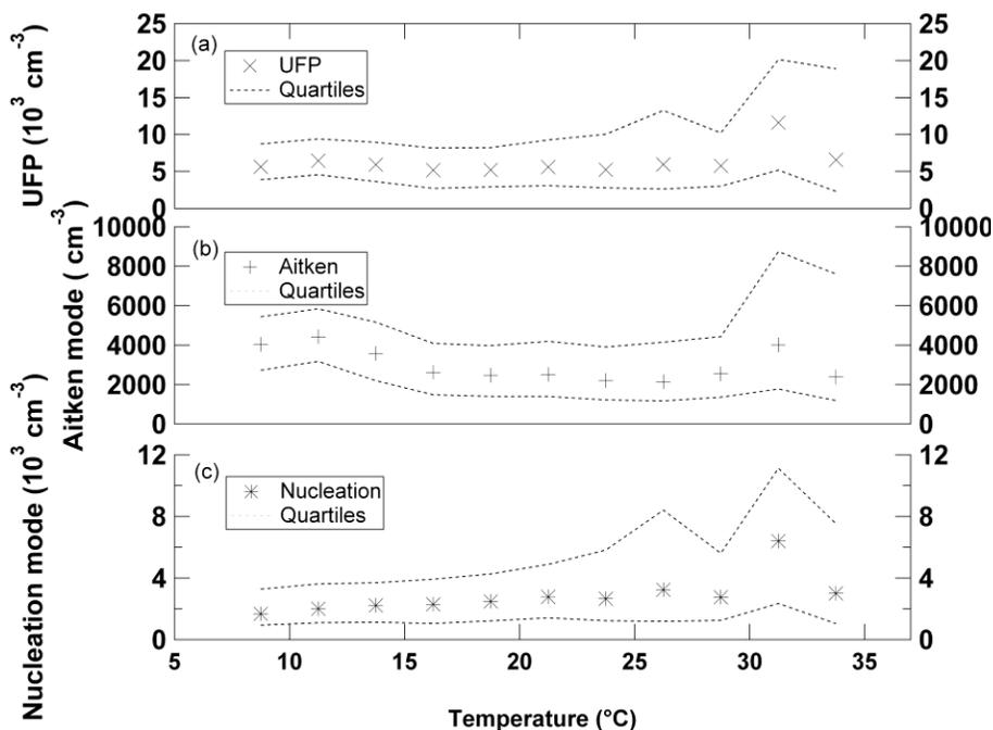
**Fig. 4.** Particle number concentrations of **(a)** ultrafine (UFP), **(b)** Aitken mode, and **(c)** nucleation mode particles and their variation as a function of temperature. The median number concentrations and the 1st and 3rd quartiles are presented.
