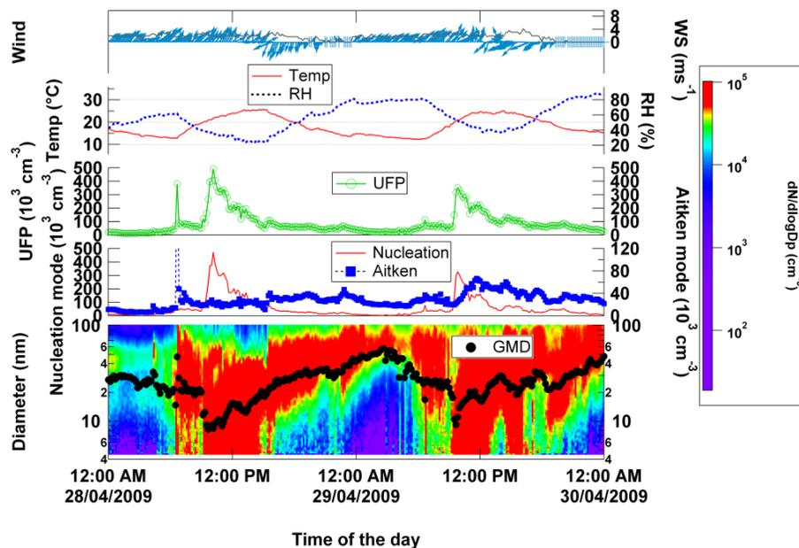
**Fig. 10.** Nucleation events observed on 28–29 April 2009. From bottom to top, the parameters are: i) Geometric median diameter (GMD); ii) Particle number concentration of nucleation and Aitken mode particles; iii) Particle number concentration of ultrafine particles (UFP); iv) Temperature and relative humidity; and v) wind direction and speed.
