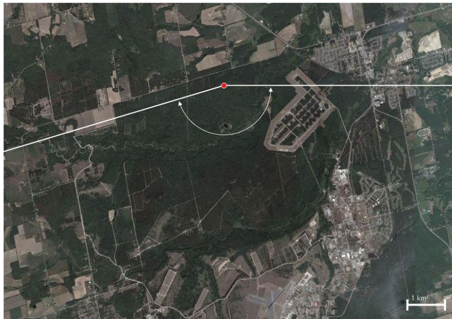
Fig. 1. Borden and surrounding area. Red dot shows tower location. Arrows show range of wind direction with adequate fetch. Photo reproduced from google.com.
