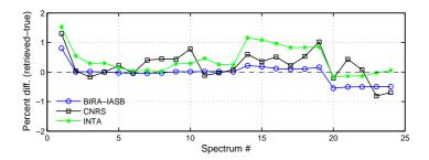
**Fig. 2.** Percent difference between retrieved and true slant column ozone values, as obtained from analysis of simulated radiances independently processed at BIRA-IASB, INTA and LAT-MOS (labeled CNRS in the plot).
