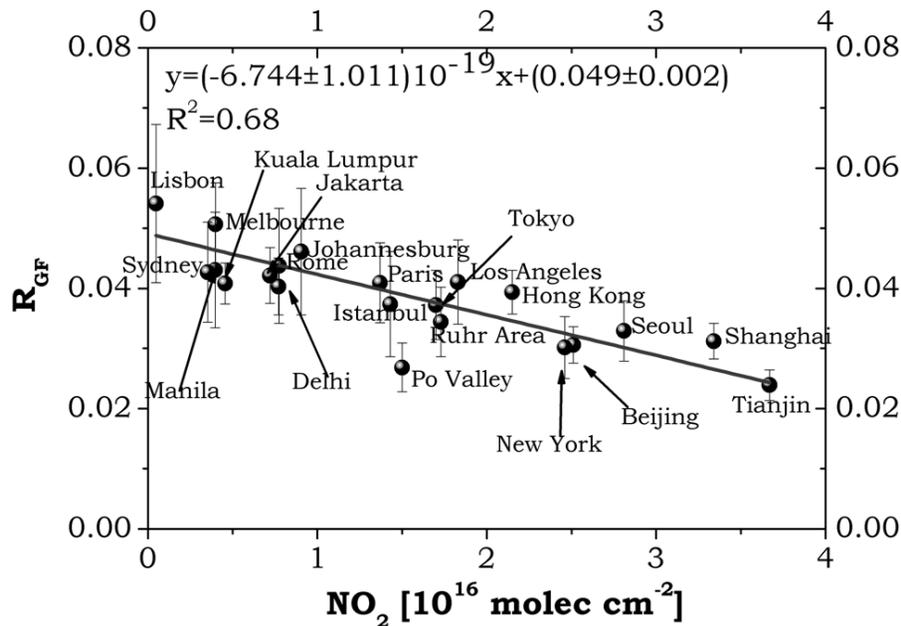
**Fig. 7.** Mean  $R_{\text{GF}}$  ratio, as a function of the  $\text{VCD}_{\text{NO}_2}$  amounts, over 21 cities/areas and for the period 2007–2008. Cities with high  $\text{NO}_2$  levels experience lower  $R_{\text{GF}}$  values while cities with low  $\text{NO}_2$  levels show higher  $R_{\text{GF}}$  ratios.
