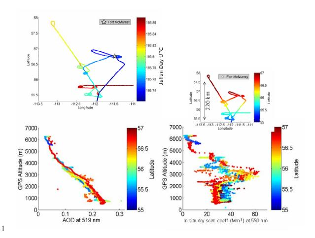
Supplementary Figure S1. Mid-visible AOD and scattering coefficient profiles near Fort McMurray during the first half of the July 3 flight. The P-3 aircraft encountered a well-mixed local pollution layer up to ~2 km GPS altitude and a long-range transport air mass above, both homogenous over >200 km.
