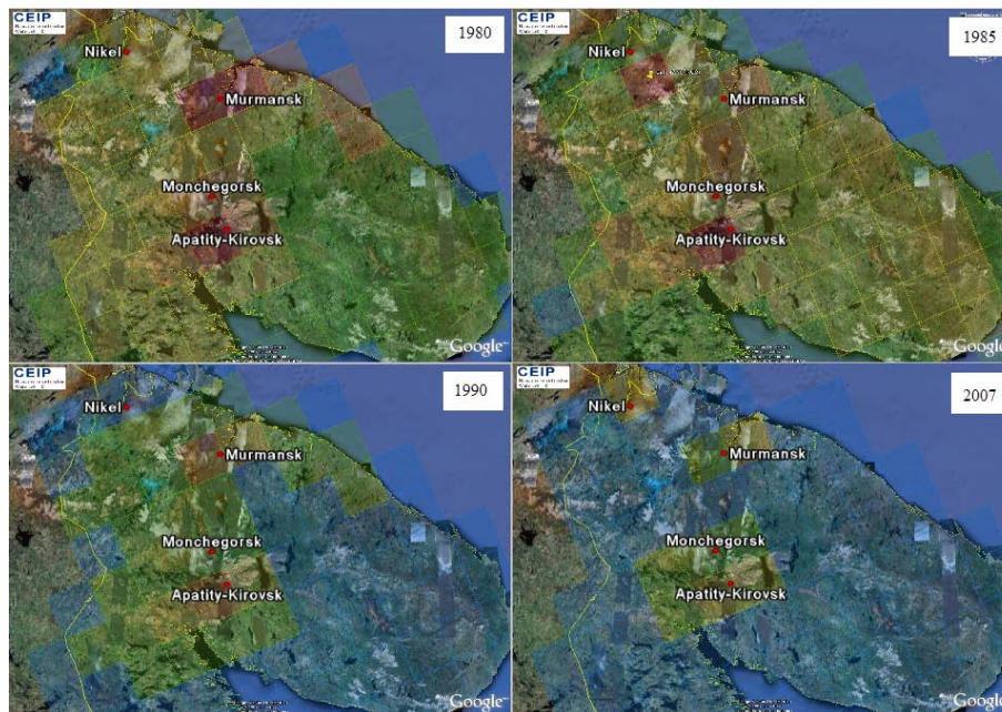
Fig. 2. The original EMEP emission for 1980–2007, WebDab status 2010. The 50 km grid cells are shown with the colours reflecting the \text{SO}_x emission: blue \leq 0.1 \text{ kT SO}_2 \text{ yr}^{-1} , green \leq 1 \text{ kT SO}_2 \text{ yr}^{-1} , yellow \leq 10 \text{ kT SO}_2 \text{ yr}^{-1} , orange \leq 100 \text{ kT SO}_2 \text{ yr}^{-1} , red > 100 \text{ kT SO}_2 \text{ yr}^{-1} . Pictures from http://www.emep.int .
