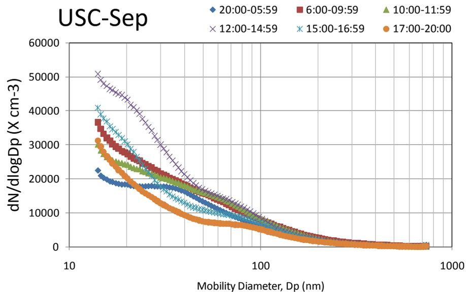
**Fig. 2b.** Average size distribution of particles during six time periods (PST) of the day at USC during September 2009.
