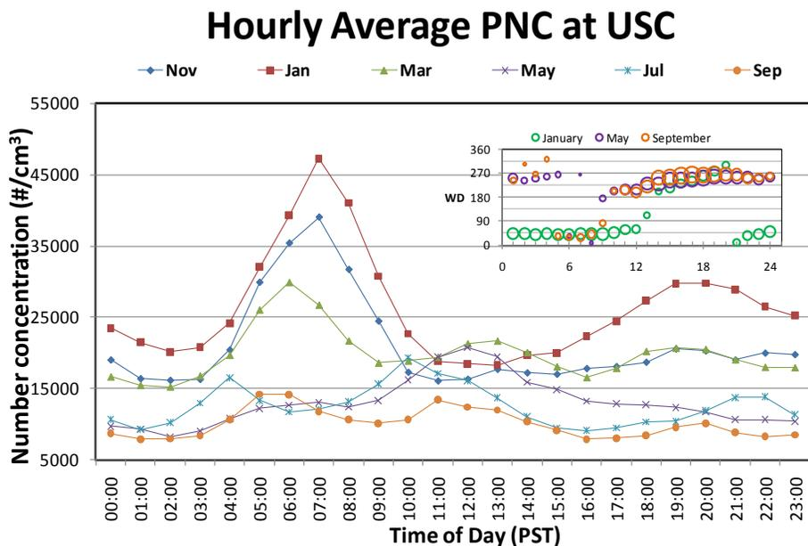
**Fig. 2a.** Hourly average particle number concentration at USC plotted for hours of the day in Pacific Standard Time (PST). The relative standard error for the hourly averages reported above was less than 2%. The inset is a plot of vector averaged wind direction (WD) with the bubble area weighed to wind speed plotted for hours of the day in PST.
