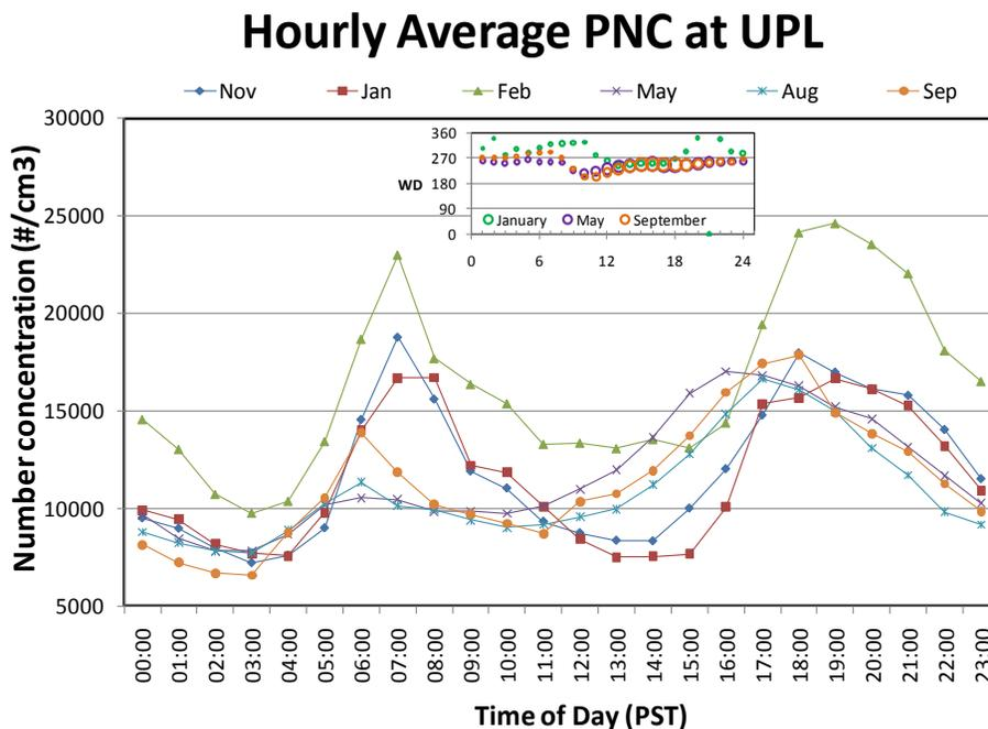
**Fig. 3a.** Hourly average particle number concentration at UPL for hours of the day in Pacific Standard Time (PST). The relative standard error for the hourly averages reported above was less than 2%. The inset is a plot of vector averaged wind direction (WD) with the bubble area weighed to wind speed plotted for hours of the day in PST.
