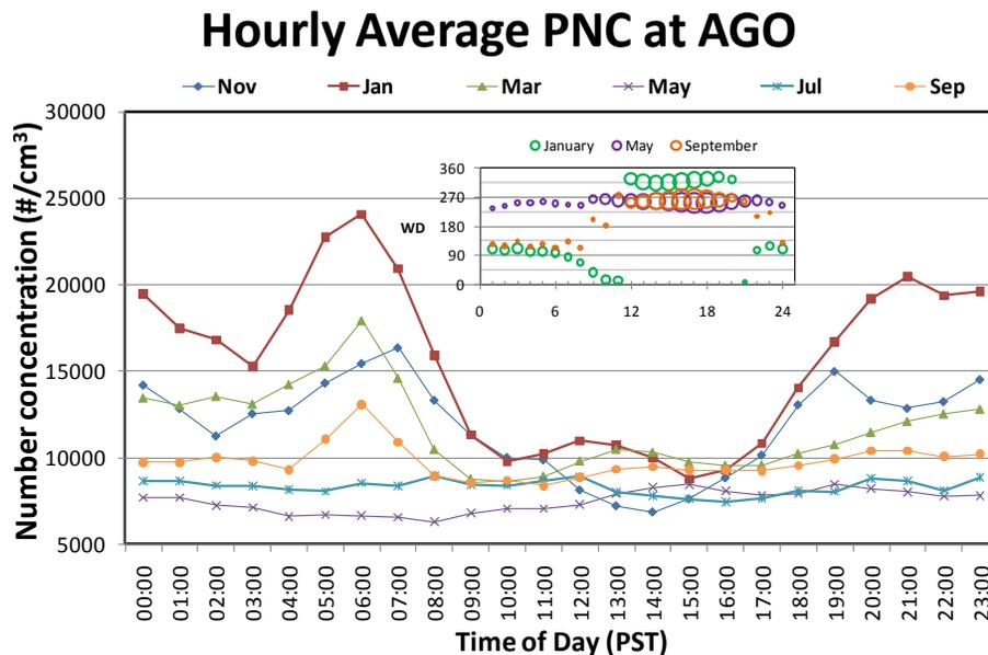
**Fig. 4a.** Hourly average particle number concentration at AGO for hours of the day in Pacific Standard Time (PST). The relative standard error for the hourly averages reported above was less than 3%. The inset is a plot of vector averaged wind direction (WD) with the bubble area weighed to wind speed plotted for hours of the day in PST.
