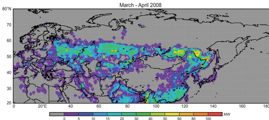
**Fig. 4.** Location of biomass fires based on the MODIS Fire Mapper (Giovanni program) for March–April of 2008. The resolution of the fire radiative power field (units of MW) is  $1^\circ \times 1^\circ$ .
