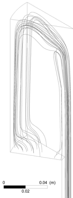
Fig. 1. A 30° radial section is used to model the flow through the inlet assembly with CFD. Air at -40^{\circ}\text{C} and 1\ \mu\text{m} diameter particles (density of 1000\ \text{kg m}^{-3} ) are introduced through the opening at the bottom of the inlet. The outer surface and the inlet pipe in the center (ending in a funnel at the top) are heated to 20^{\circ}\text{C} . Trajectories of the 1\ \mu\text{m} particles are depicted as grey lines.
