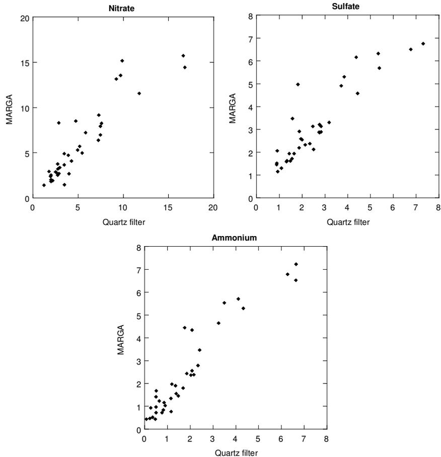
**Fig. 1.** Comparison between daily average concentrations ( $\mu\text{g}/\text{m}^3$ ) of nitrate, sulfate and ammonium as obtained by the MARGA and co-located quartz filter samples.
