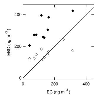
**Fig. 3.** Scatter plot of EBC concentration at Trinidad Head calculated with  $\sigma^*$  equal to 10 m<sup>2</sup> g<sup>-1</sup> (full diamonds) and 20 m<sup>2</sup> g<sup>-1</sup> (empty diamonds) versus the average EC concentration at the IMPROVE sites; black line indicates the 1:1 ratio.
