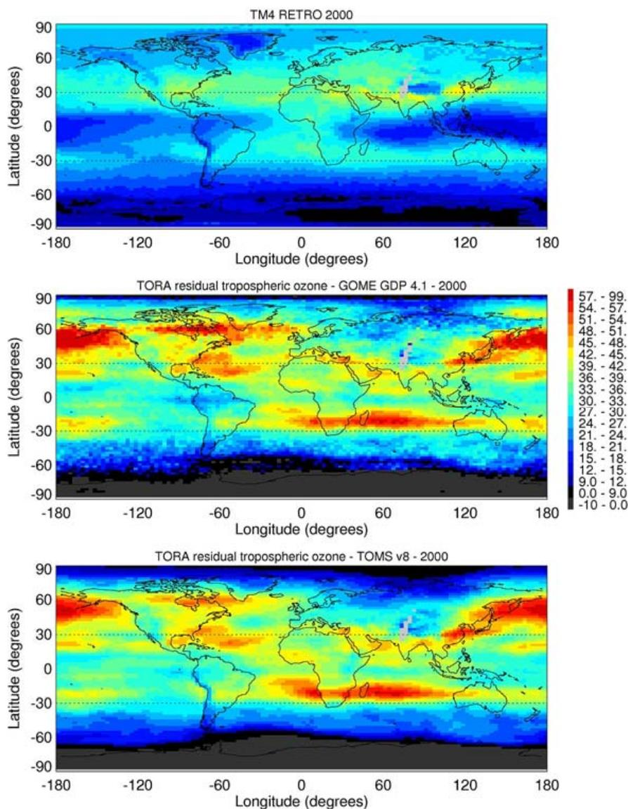
**Fig. 6.** Global mean total tropospheric O<sub>3</sub> columns (TTOC's) for the year 2000 in DU. Upper panel: TM4 simulated TTOC from the RETRO-project reanalysis simulations (RETRO, 2007). Middle panel: TORA O<sub>3</sub> residuals from GDP v4.1 total O<sub>3</sub> columns minus TM5 GOME assimilated stratospheric O<sub>3</sub> columns. Lower panel: as middle panel but using TOMS v8 instead of GOME GDP v4.1 total O<sub>3</sub> columns
