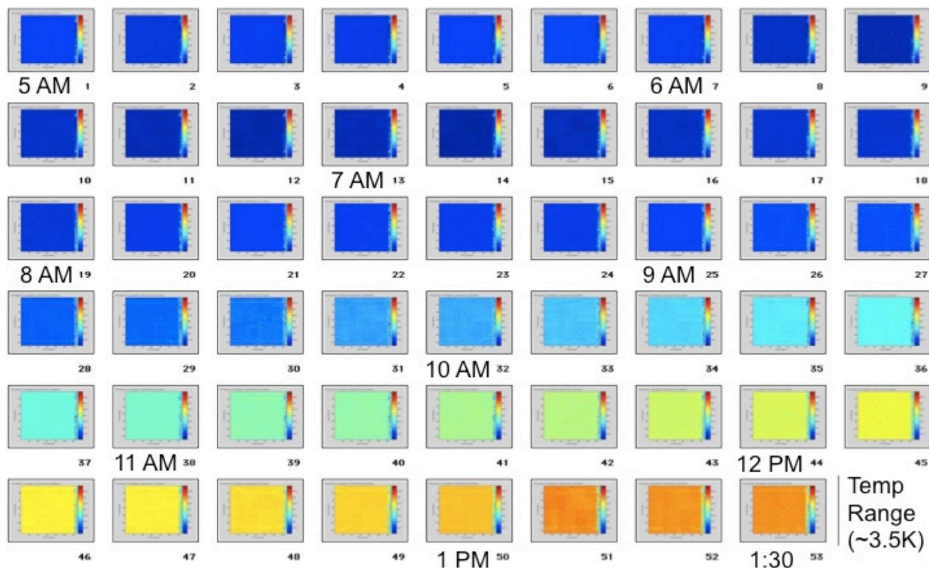
**Fig. 13.** Consecutive 10 min interval  $128 \times 128$  detector element frames of 600-m level (800 hPa) atmospheric temperature retrieved from GIFTS sky-viewing radiance observations at Logan UT on 13 September 2006.
