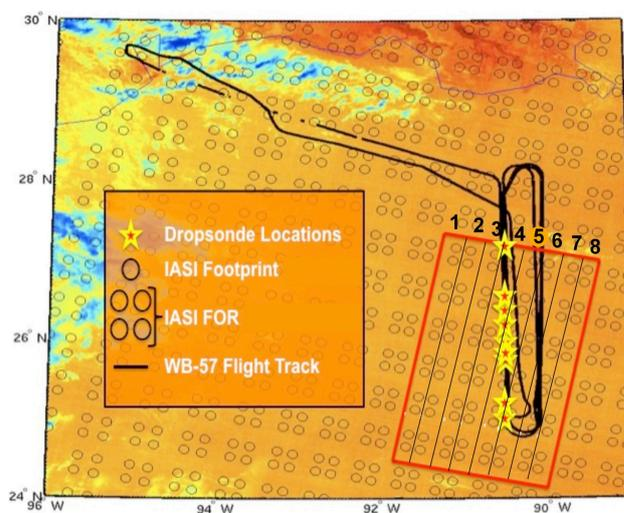
**Fig. 5.** The location of the IASI footprints, the aircraft flight track, and the dropsonde locations, superimposed upon a 10–12  $\mu\text{m}$  infrared cloud image obtained with the IASI at 15:50 UTC on 29 April 2007. The red box delineates the validation area of interest.
