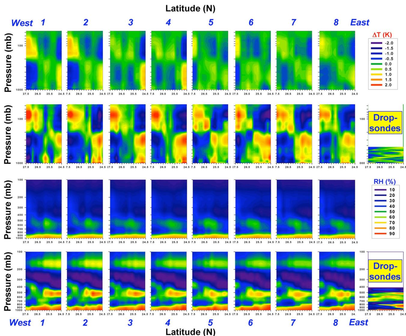
**Fig. 7.** North-South vertical cross-sections of atmospheric temperature deviation from the mean (upper two panels) and moisture relative humidity (lower two panels) for the eight columns of IASI footprints shown in Fig. 5. The upper panel for each variable corresponds to retrievals from the IASI simulated multi-spectral (ABI) radiance observations, whereas the bottom panel corresponds to retrievals obtained from full spectral resolution IASI radiances.
