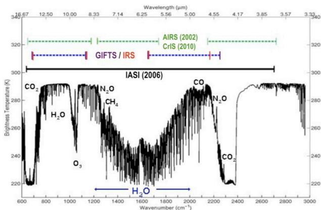
**Fig. 8.** Spectral coverage of various ultra-spectral sounding instruments.
