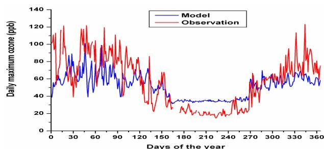
**Fig. 2c.** Comparison between modeled and observed daily maximum ozone concentrations for the year 2003 at Pune.
