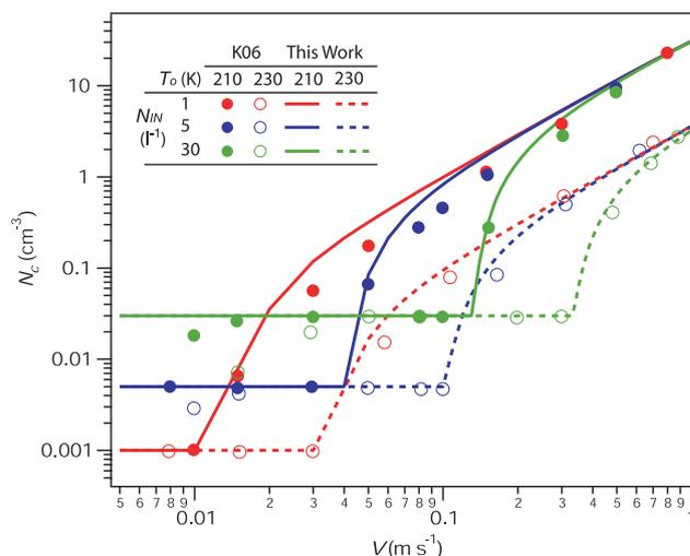
**Fig. 5.** Comparison of new parameterization (lines) against the formulation of Kärcher et al. (2006) (symbols). Simulations shown are for  $T_o=210$  K, 230 K,  $p=22\,000$  Pa, and,  $\alpha_d=0.5$ .  $N_{\text{IN}}$  was set to 1, 5, and  $30 \text{ l}^{-1}$ , and,  $S_h$  to 1.3.
