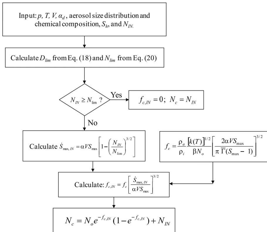
Fig. 2. Parameterization algorithm.
