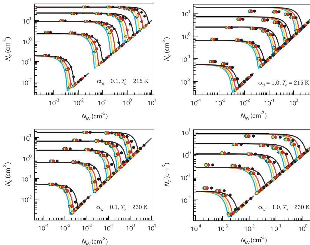
**Fig. 3.**  $N_c$  vs.  $N_{IN}$  for all simulation conditions of Table 1. Lines represent parameterization results and symbols correspond to parcel model simulations. Symbols are colored by  $S_h$ , being 1.1 (blue), 1.2 (yellow), 1.3 (red), and 1.4 (black).  $V$  is equal to 0.04, 0.2, 0.5, 1, and 2  $\text{m s}^{-1}$ , from bottom to top lines in each panel, respectively.
