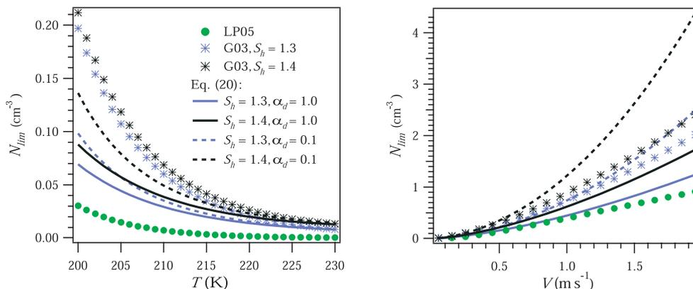
**Fig. 6.**  $N_{\text{lim}}$  vs.  $T$  at  $V=0.1 \text{ m s}^{-1}$  (left panel) and  $N_{\text{lim}}$  vs.  $V$  at  $T=215 \text{ K}$  (right panel), calculated using the parameterizations of Gierens (2003, G03), Liu and Penner (2005, LP05), and Eq. (20).
