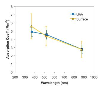
**Fig. 7.** Comparison of spectral absorption data from a commercial aethalometer located on the ground with an airborne absorption photometer flying within the mixed layer (<400 m a.s.l.) on 23 March 2006.
