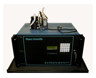
**Fig. 3.** Absorption photometer developed for deployment on AUAVs sitting atop the original, commercial, 19" rack-mount instrument (Magee Scientific AE-31 Aethalometer).
