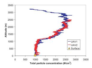
**Fig. 4.** Comparison of total particle concentration measurements collected from two UAVs launched within 15 min of each other on 28 March 2006. The yellow triangle was the average particle concentration measured at the ground station during the same period.
