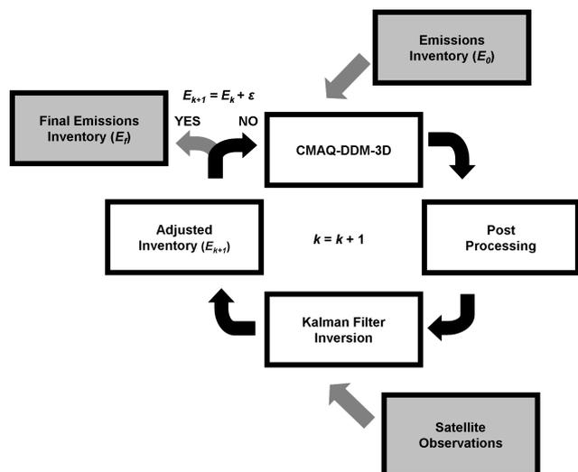
**Fig. 3.** Outline of the presented inverse method. The iterative process is used to overcome nonlinearities in the relationship between NO<sub>x</sub> emissions and NO<sub>2</sub> concentrations. The convergence criteria ( $E_{k+1} = E_k + \epsilon$ ) can vary with application, but  $0.001 < |(E_{k+1} - E_k)/E_k|$  was used here.
