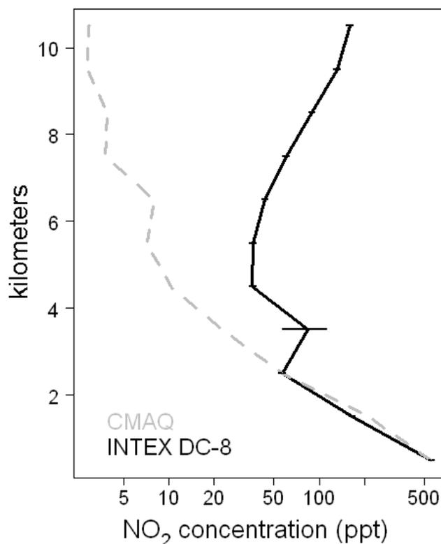
**Fig. 7.** Vertical distribution of NO<sub>2</sub> concentrations observed by NASA INTEX DC-8 flights over the eastern United States compared to model predictions matched in space and time. Error bars denote 99% confidence interval of the mean, assuming that observations are drawn from a normally distributed population. For more measurement details, see Bertram et al. (2007), Supporting Online Material, Fig. S6.
