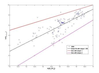
**Fig. 8.** Logarithm of the number concentration of 6–10 nm particles  $(N_{6-10})$  versus logarithm of the sulphuric acid concentration for all 4 days. Linear fit to the data by the method of least squares and lines corresponding relationships  $N_{6-10} - [\text{H}_2\text{SO}_4]^2$  and  $N_{6-10} - [\text{H}_2\text{SO}_4]^2$  are shown.
