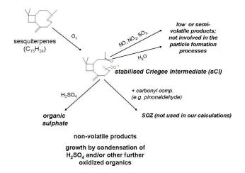
Fig. 9. Schematic picture of the nucleation mechanism by activation of organic molecules.
