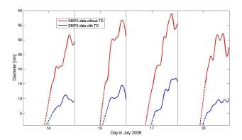
**Fig. 5.** Evolution of geometric mean diameter (solid line) and linear fit (dashed line) of nucleation mode without and with TD during selected nucleation event days (x-axis from midnight to midnight for each day).
