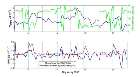
**Fig. 11.** Calculated mass and wind direction for 4 selected event days (upper plot); mass change and contribution by sulfuric acid (lower plot). The light blue vertical line indicates for each day the time when new particle formation was observed at the NWR.
