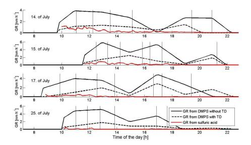
**Fig. 6.** Detected growth rates (GR) of the mean nucleation mode diameter from the TDMPS data without and with TD; calculated GR through sulfuric acid. The light vertical black lines indicate the times, when the mean nucleation mode particles reached diameters of 5, 10, 15, 20, 25, 30 and (35) nm.
