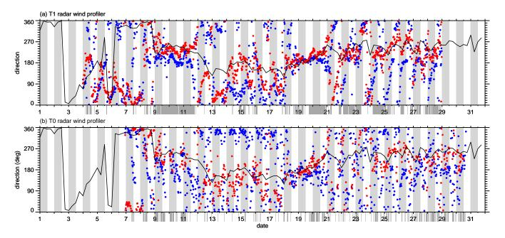
**Fig. 17.** Wind direction measured by radar wind profiles at the 400 m (blue dots) and 1500 m (red dots) a.g.l. range gates at the (a) T1 and (b) T0 sites. Black line denotes the 500 hPa-level wind speed and direction from the GFS grid point closed to Mexico City and gray shading denotes nighttime periods. Gray shading along the x-axis denotes periods with directions between 195 and 255 degrees that are favorable for transport from Mexico City to the T1 and T2 sampling sites.
