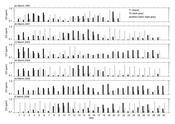
**Fig. 19.** Daily afternoon CO concentrations simulated by WRF-chem and averaged between 18:00 and 00:00 UTC over the T1 (black), T2 (dark gray), and Santa Ana (light gray) sites. Santa Ana located in the southern basin (Fig. 2b).
