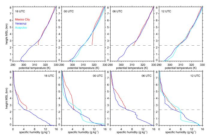
**Fig. 15.** Average potential temperature and specific humidity profiles at 6-h intervals from the Mexico City, Veracruz, and Acapulco rawinsondes during the field campaign. The dashed line denotes the elevation of the Mexico City basin.
