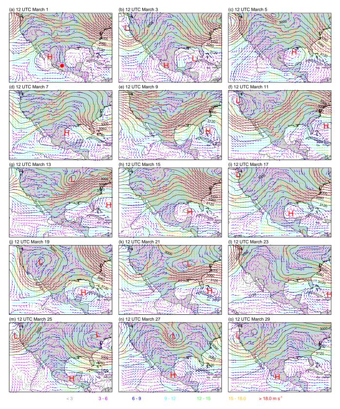
**Fig. 3.** Winds (arrows) and geopotential heights (contours) at 700 hPa at 12:00 UTC for every-other day during the field campaign period during March 2006. Red dot in (a) denotes Mexico City. Contour intervals of 30 m.
