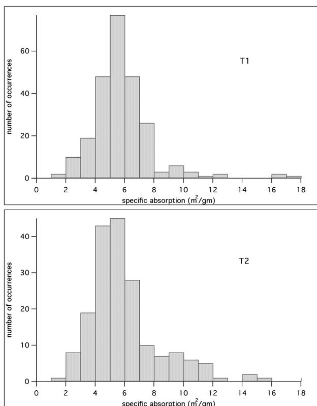
**Fig. 1.** Histograms of specific absorption of EC at 870 nm at T1 (top) and T2 (bottom). The histogram for T1 represents 250 h of data while that for T2 represents 188 hours.
