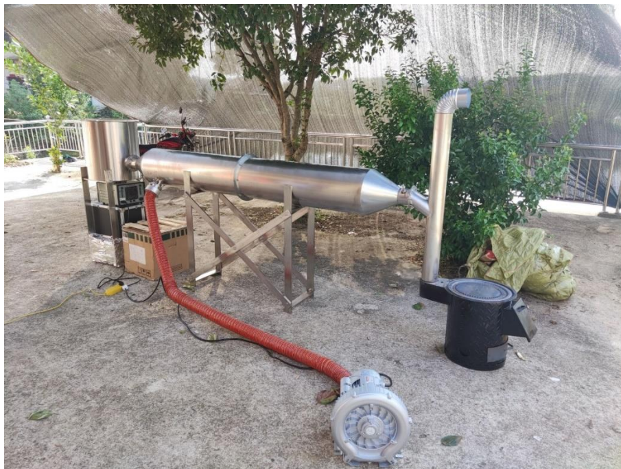
22 23 Figure S2. A photo of the apparatus used in our work to collect aerosol particles emitted by 24 domestic coal and biofuel burning.
