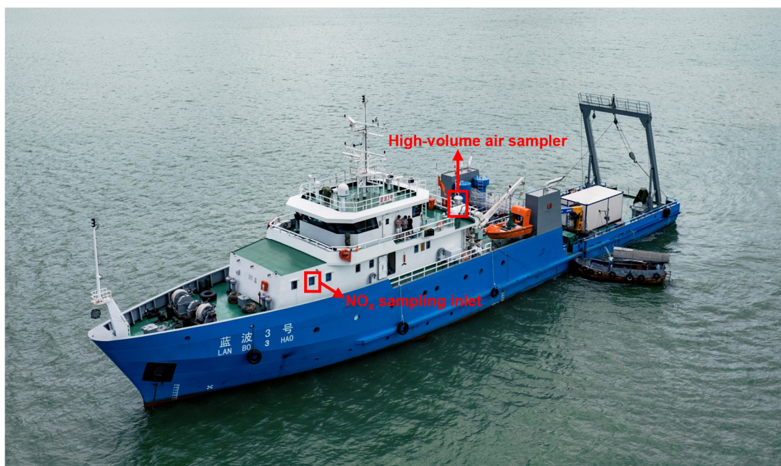
Figure S6. Photograph of the shipboard aerosol sampling configuration during the cruise campaign. Red boxes and arrows indicate the location of the high-volume air sampler on the upper deck outside the bridge and the nearby NO x sampling inlet on the lower deck, illustrating their close proximity and the basis for using NO x as an operational screen for ship-exhaust influence.
