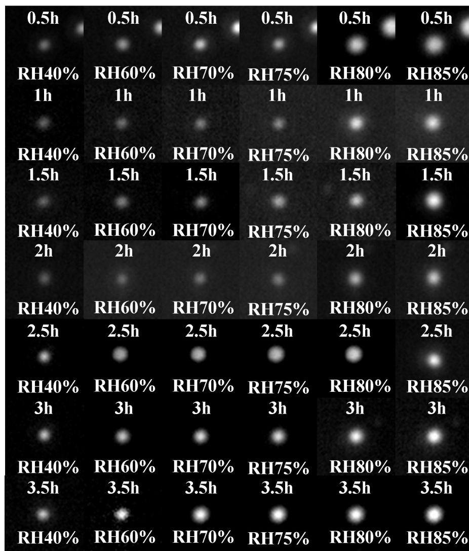
Figure S7. In situ dark-field images of NaCl single nano-particle (150 nm) with the reaction time of from 0.5 h to 3.5 h at humidification process.
