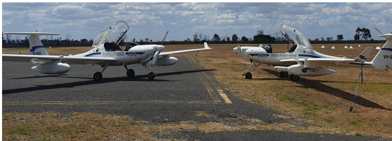
Fig. S1. The two Diamond Aircraft HK36TTC-ECO Dimonas owned and operated by Airborne Research Australia. The aircraft on 245 the left is the remote sensing aircraft, and the aircraft on the right is the in-situ aircraft.
