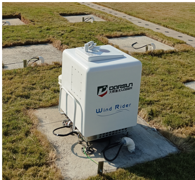
Figure 1. Installation photograph of the wind lidar.
