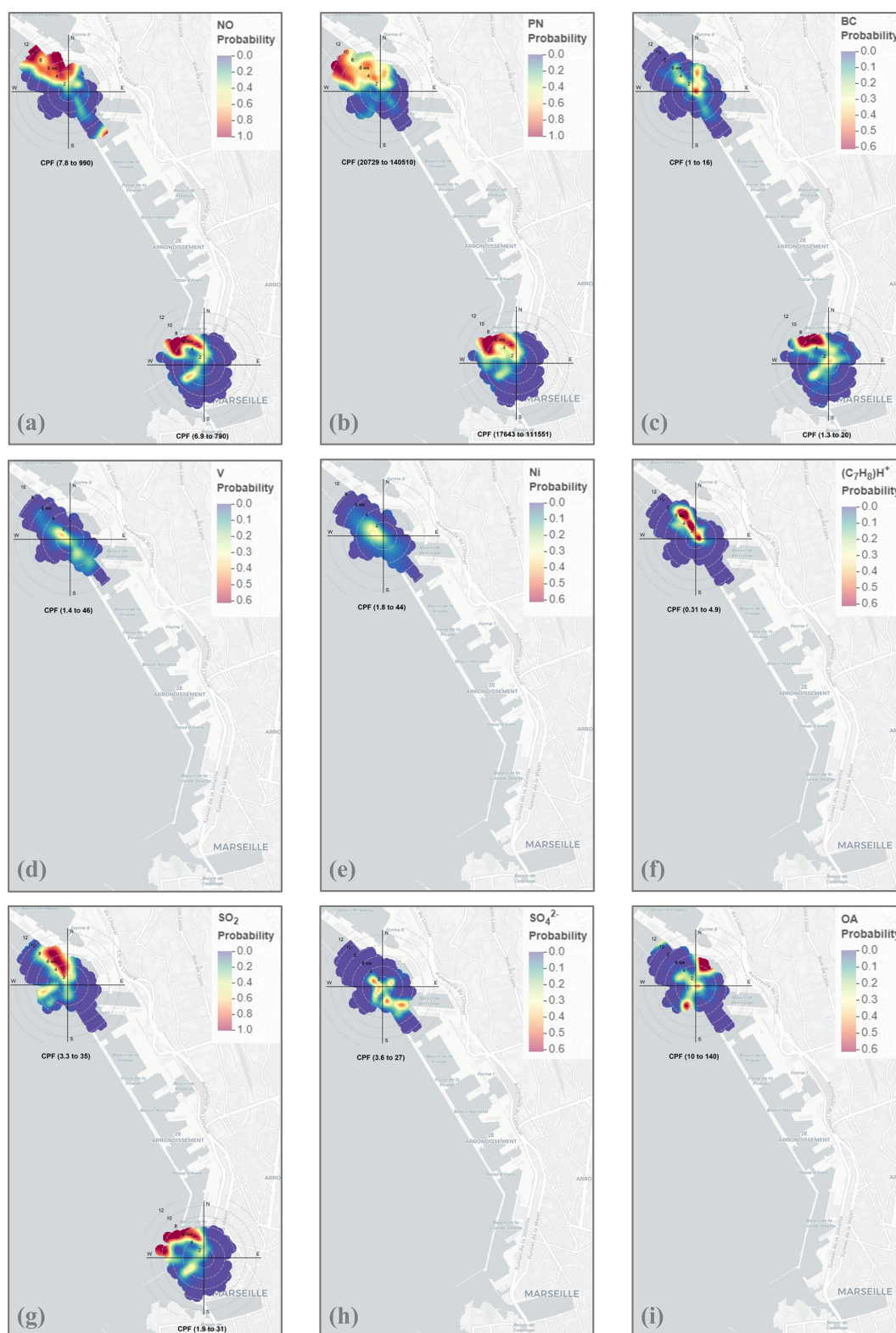
Figure 4. Conditional bivariate probability function (CBPF) computed for (a) NO, (b) PN, (c) BC, (d) V, (e) Ni, (f) toluene (NMVOC), (g) SO_2 , (h) SO_4^{2-} , and (i) OA during the campaign at the PEB and MAJOR stations. The radial axis indicates wind speed in m s^{-1} , and the colour bar indicates the probability of a species being above the 80th percentile of the compound. Maps taken from © OpenStreetMap contributors 2023 © CARTO. Distributed under the Open Data Commons Open Database License (ODbL) v1.0.
