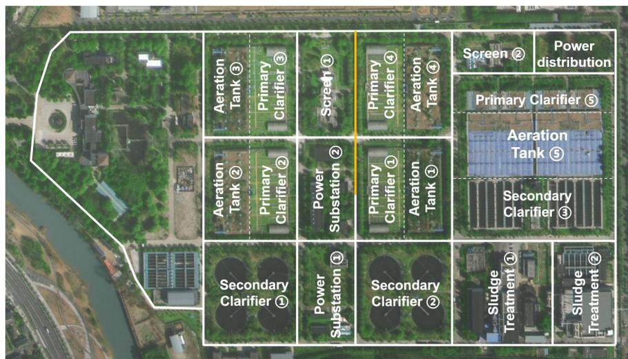
**Figure 1.** Distribution of the WWTP functional areas. The yellow mark represents the simulated location of the line source. Solid lines show the roads measured by the mobile vehicle. Map data are from Esri.
