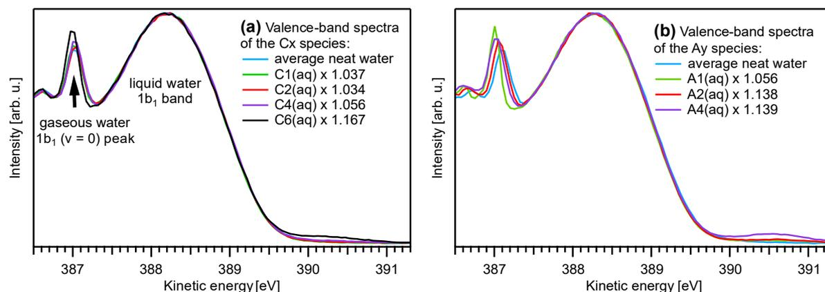
**Fig. S2:** Analysis of valence-band intensity for single-species aqueous solutions: (A)  $C_x(aq)$  and (B)  $A_y(aq)$ ; A6 is not shown as this species was measured in a different experimental campaign. Each solution's PE spectrum was scaled until the intensity of the liquid-water  $1b_1$  band matched that of an average neat-water spectrum. Scaling factors to achieve this are indicated in the legend.
