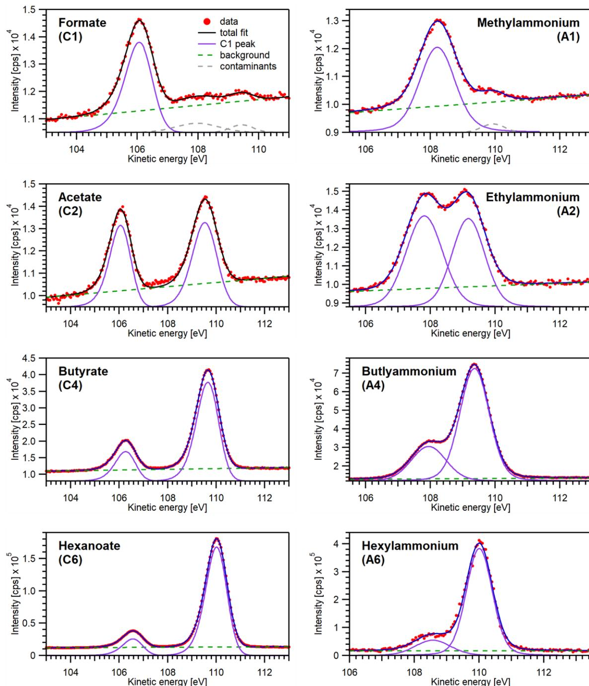
**Fig. S4:** PE spectra (red dots) of the single-component solutions together with the total fits (black) and individual peak components (purple). Dashed grey lines indicate contributions from contaminants and green dashed lines are the linear background. Intensities of the C6 and A6 spectra are scaled to account for the different BDA slit setting for the former and the overall intensity difference due to experimental settings for the latter.
