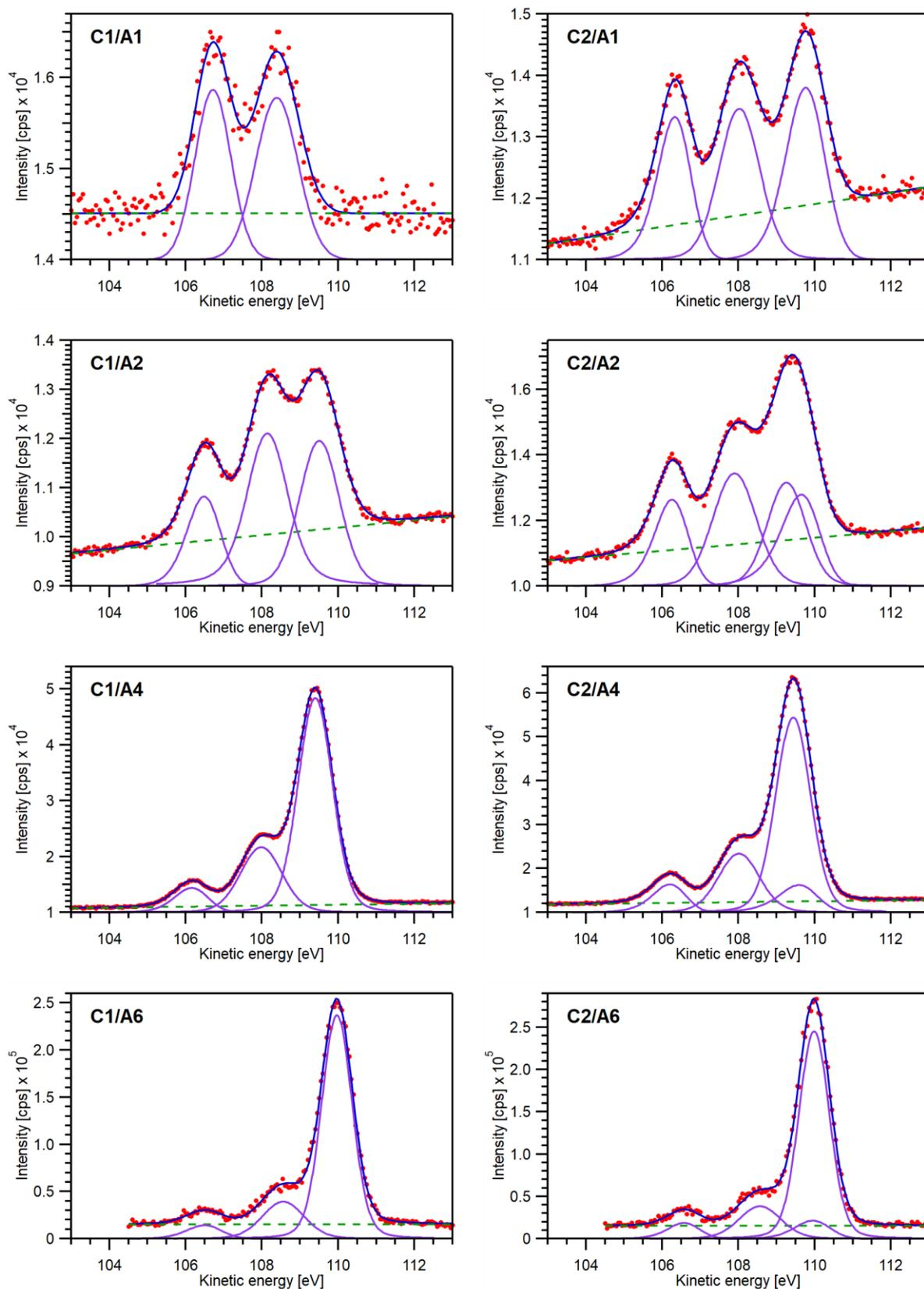
**Fig. S5:** PE spectra (red dots) of the mixed-component solutions  $C_x/A_y$  ( $x = 1, 2$  and  $y = 1, 2, 4, 6$ ) together with the total fits (black), individual peak components (purple), and the linear background (green dashed line). Intensities of the spectra for the C1/A1, C1/A6, and C2/A6 mixtures are from a different measurement campaign. These spectra are scaled according to a factor to match a reference measurement of C1 in each campaign.
