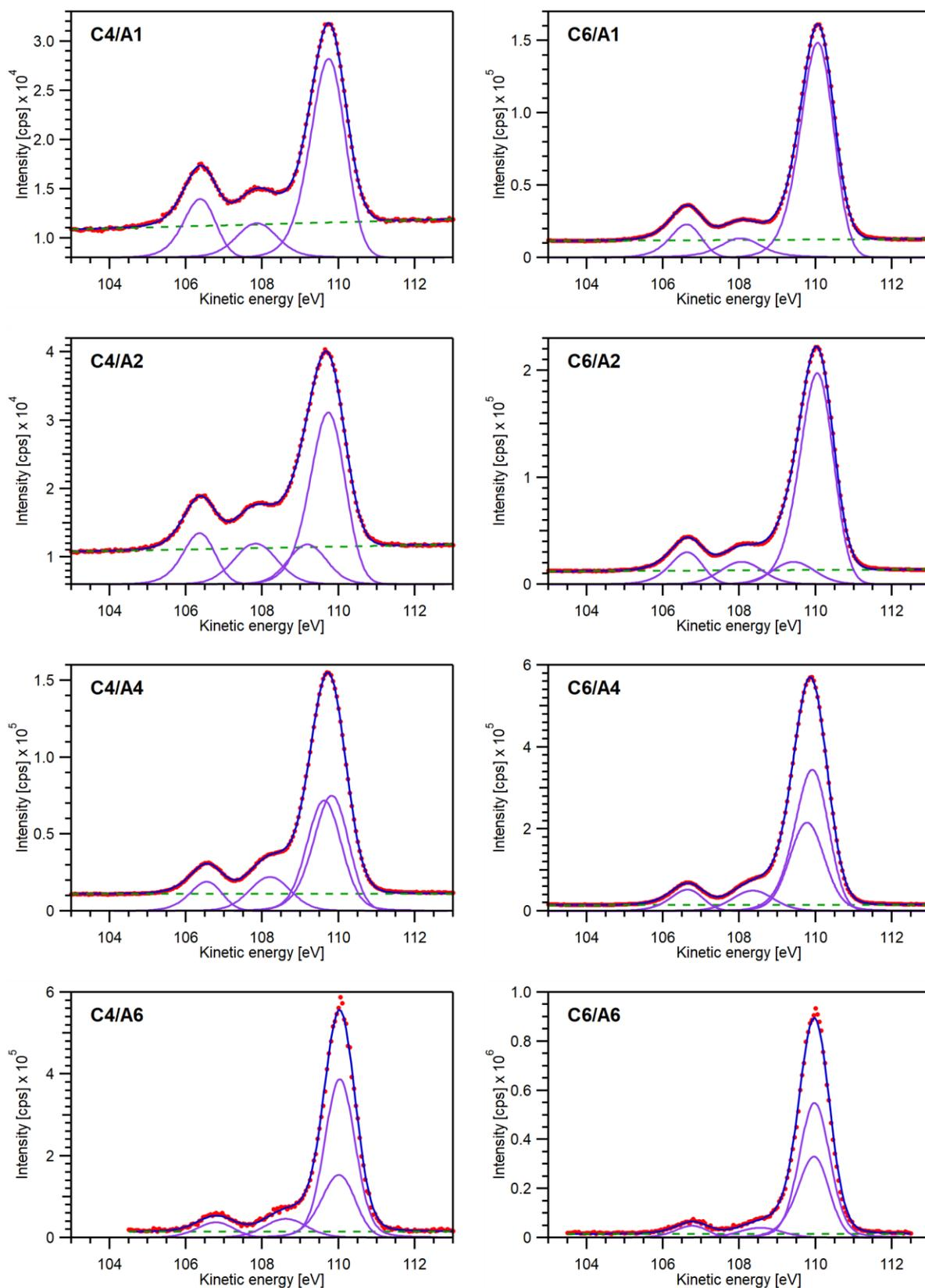
**Fig. S6:** PE spectra (red dots) of the mixed-component solutions  $C_x/A_y$  ( $x = 4,6$  and  $y = 1,2,4,6$ ) together with the total fits (black), individual peak components (purple), and the linear background (green dashed line). Intensities of the spectra for the C4/A6 and C6/A6 mixtures are from a different measurement campaign. These spectra are scaled according to a factor to match a reference measurement of C1 in each campaign.
