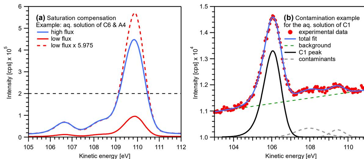
**Fig. S1:** Treatment of experimental issues: (a) signal saturation and (b) contaminant signals.
