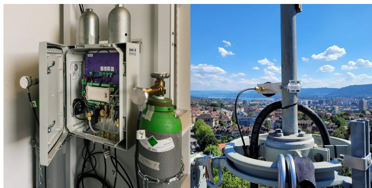
Figure A1. Examples of the CO 2 sensor's typical installation in the ZICOS-M sensor network in the city of Zurich. The photograph on the left was taken by Pekka Pelkonen from ICOS RI.
