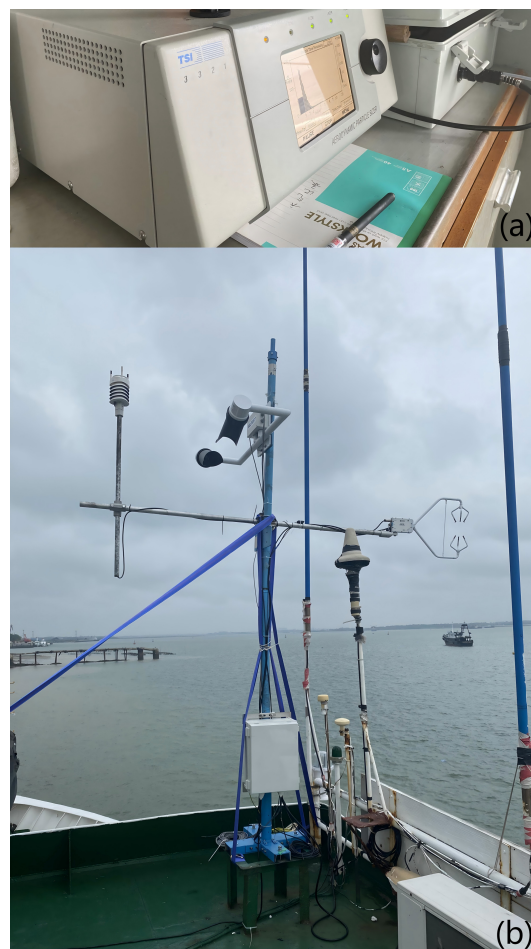
Figure 1. The total view of (a) the Model 3321 APS spectrometer and (b) the automatic meteorological observation system.
