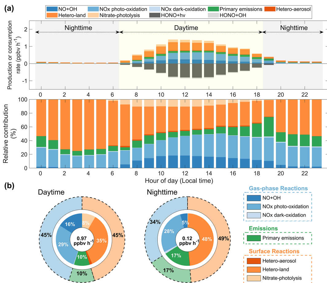
Figure 5. Attribution of mechanisms of HONO formation in coastal Fujian in May 2024. Panel (a) shows the diurnal variations in the absolute and relative contributions of seven production and two consumption reactions to the HONO chemical budget. Panel (b) illustrates the contribution of the seven production reactions to daytime and nighttime HONO formation during the study period. The total production rates are labelled in the middle of the pie charts.
