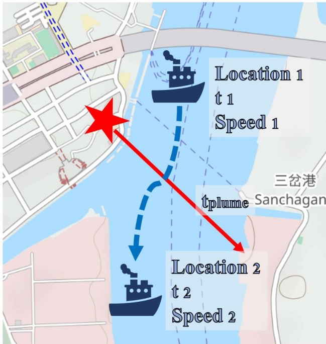
Figure S13. Schematic Diagram of the Matching Between Ship AIS Data and SO 2 -rich plume signals. With ship's positions at two locations (Location 1 and Location 2 ) are shown along with their respective timestamps ( t_1 and t_2 ) and speed (Speed 1 and Speed 2 ). The bidirectional arrows indicate the light path of DOAS. t_{\text{plume}} indicates when the SO 2 -rich plume appeared. Base map: © OpenStreetMap contributors 2025. Distributed under the Open Data Commons Open Database License (ODbL) v1.0.
