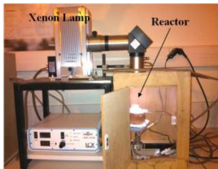
Fig. S1 Home-made Pyrex jacketed cylindrical photo-reactor.
