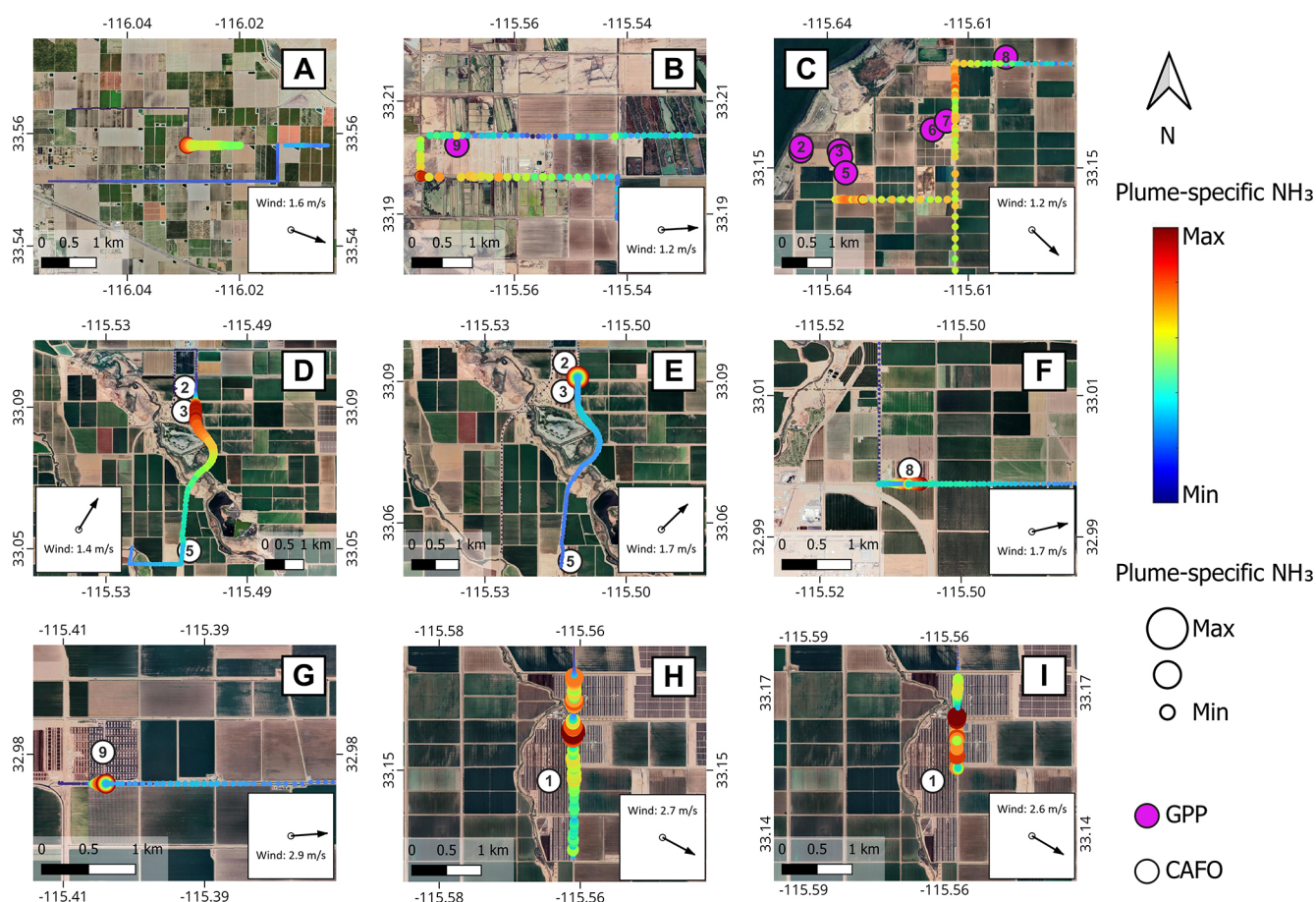
Figure 9. Maps of individual ground-level \text{NH}_3 plumes (A–I), as defined in Fig. 8, measured by the mobile platform. The color bar and marker sizes represent the plume-specific \text{NH}_3 range, where blue and red correspond to the minimum and maximum \text{NH}_3 values within each panel, respectively. Because scaling is performed separately for each plume, colors and marker sizes highlight spatial patterns within plumes but are not comparable across panels. Absolute concentrations and cross-plume comparisons are provided in Figs. 8 and 10. Average wind speed and direction were calculated from the nearest HRRR grid cells. Base imagery © Google Earth 2025.
