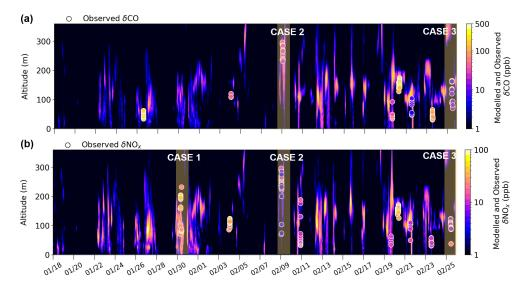
Figure 6. Comparison of modelled (CTRL) power plant and observed trace gas enhancements above background (> 30 m) for (a)  $\delta$ CO (ppb) and (b)  $\delta$ NO<sub>X</sub> (ppb) at the closest grid cell to the UAF Farm. Observed plume enhancements are shown as circles (ppb). Cases discussed in the main text are highlighted.
