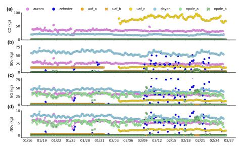
**Figure A2.** Emissions of (a) CO, (b) SO<sub>2</sub>, (c) NO, and (d) NO<sub>2</sub> (kg) for each power plant stack (indicated above panel a) as a function of time during ALPACA-2022. Averages of 3 h are shown for clarification of the data points, but 1 h data are used in the modelling study.
