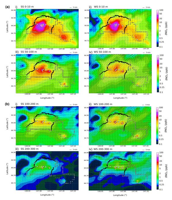
**Figure C2.** Spatial maps of total power plants and surface-emitted tracer enhancements (CTRL simulation) for (i) SS and (ii) WS conditions for CO (ppb) at (a) 0–10 m (top), 50–100 m (lower), and (b) 100–200 m (top) and 200–300 m (lower). Wind vectors (black arrows) indicate average wind direction (°) and wind speeds (m s<sup>-1</sup>) simulated by EPA-WRF.
