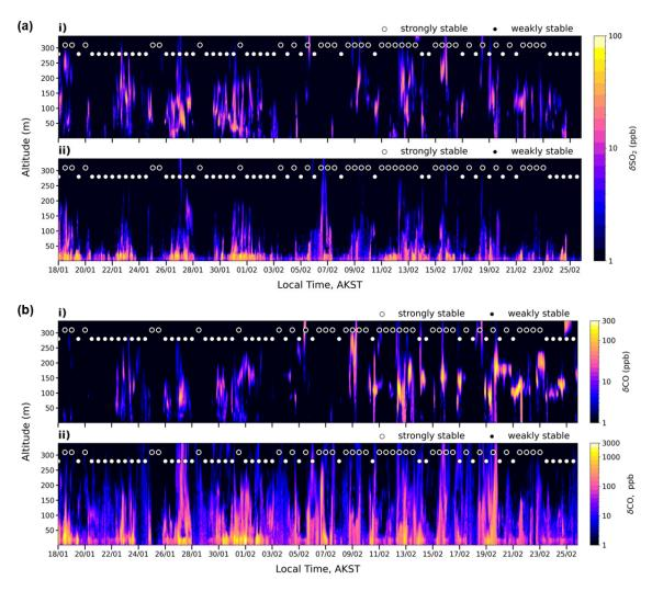
Figure C3. (a) Total power plants (i) and surface-emitted (ii) tracer enhancements (CTRL simulation) as a function of altitude and time for (a) SO<sub>2</sub> (ppb) at Hamilton Acres and (b) CO (ppb) at the UAF Farm. The WS and SS stability regimes are indicated every 12 h.
