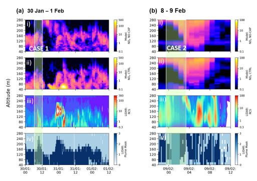
**Figure D3.** (i, ii) Simulated power plant  $NO_x$  tracers (ppb) as a function of altitude and time for the NO-CAP and CTRL simulations, respectively. (iii) Aerosol backscatter coefficient observed by wind lidar observations and (iv) lidar plume mask (described in Appendix D), for (a) 30 January to 1 February in the Downtown area (case 1, highlighted by the white box) and (b) 8 to 9 February at the UAF Farm (case 2, highlighted by the white box).
