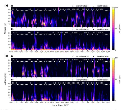
**Figure 5.** (a) Modelled (CTRL) SO<sub>2</sub> tracer (ppb) as a function of altitude (m) and local time (AKST, hours) for (i) total power plant emissions and (ii) total surface emissions (a) Downtown and (b) at the UAF Farm. The WS and SS surface stability regimes are indicated every 12 h by filled (solid) and unfilled (open) circles, respectively.
