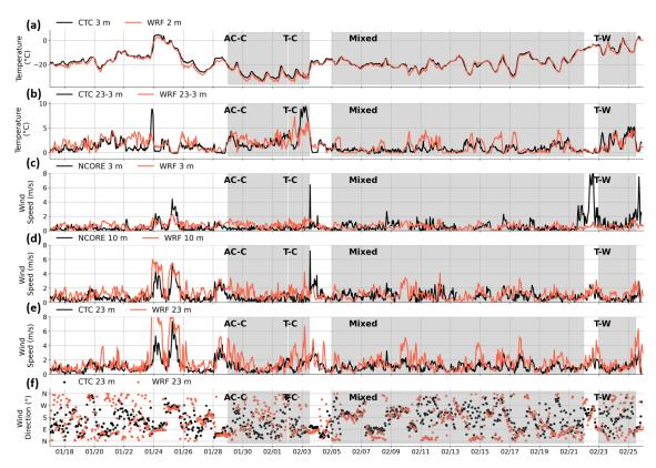
**Figure B1.** Time series of surface and near-surface temperatures (°C), temperature gradients (dT, °C), wind speeds ( $m s^{-1}$ ), and directions (°) Downtown compared to EPA-WRF (red) for available observations (black) up to 23 m altitude during ALPACA-2022.
