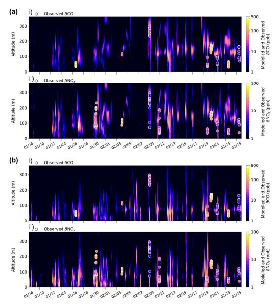
**Figure D1.** Comparison of modelled power plant and observed trace gas enhancements above background (> 30 m) for (a) NO-CAP and (b) NO-RISE and (i)  $\delta$ CO (ppb) and (ii)  $\delta$ NO<sub>x</sub> (ppb) at the closest grid cell to the UAF Farm. Periods with available observations are shown. Observed plume enhancements are shown as circles (ppb).
