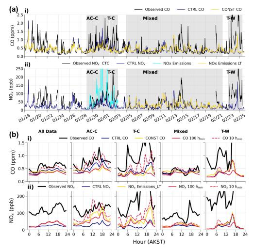
**Figure E1.** (a) Total modelled surface and power plant tracers as a function of time between 0–5 m for CTRL and selected sensitivity simulations described in Table 2 compared to available surface observations, at HA for (i) CO and (ii)  $NO_x$ . (b) Average diurnal cycles at HA for observations (black) and model simulations (colours as in a) for (i) CO and (ii)  $NO_x$ , averaged over all data and for events AC–C, T–C, Mixed, and T–W.
