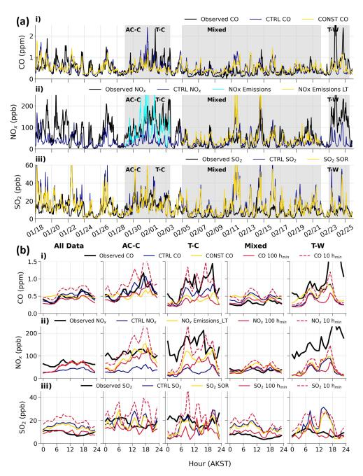
**Figure 9. (a)** Total modelled surface and power plant tracers (in ppb) as a function of time between 0–5 m for CTRL and selected sensitivity simulations described in Table 2 compared to available surface observations Downtown for (i) CO, (ii)  $NO_x$ , and (iii)  $SO_2$ . (b) Diurnal cycles, Downtown, for observations (black) and model simulations (colours as in **a**), averaged over all data (left) and over events AC–C, T–C, Mixed, and T–W. CONST CO signifies the CONST-EM sensitivity run.
