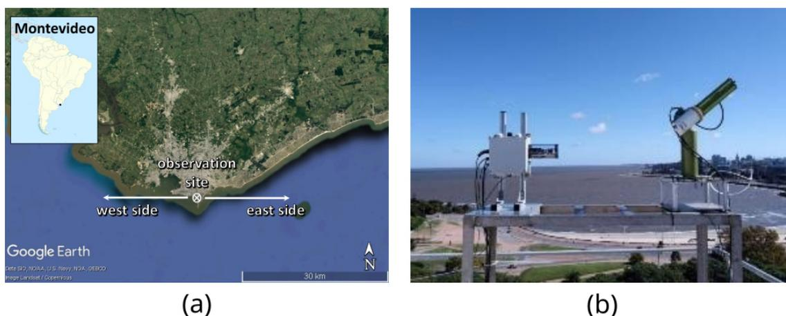
**Figure 1.** (a) Map (© Google Earth 2023) of Montevideo and the geometry used for the MAX-DOAS measurements. The observation site is located at the Faculty of Engineering. The spectrometer scans a vertical plane from east to west at several elevations. (b) Picture of the MAX-DOAS instrument (left) and the CIMEL sun photometer (right) on the roof of the building.
