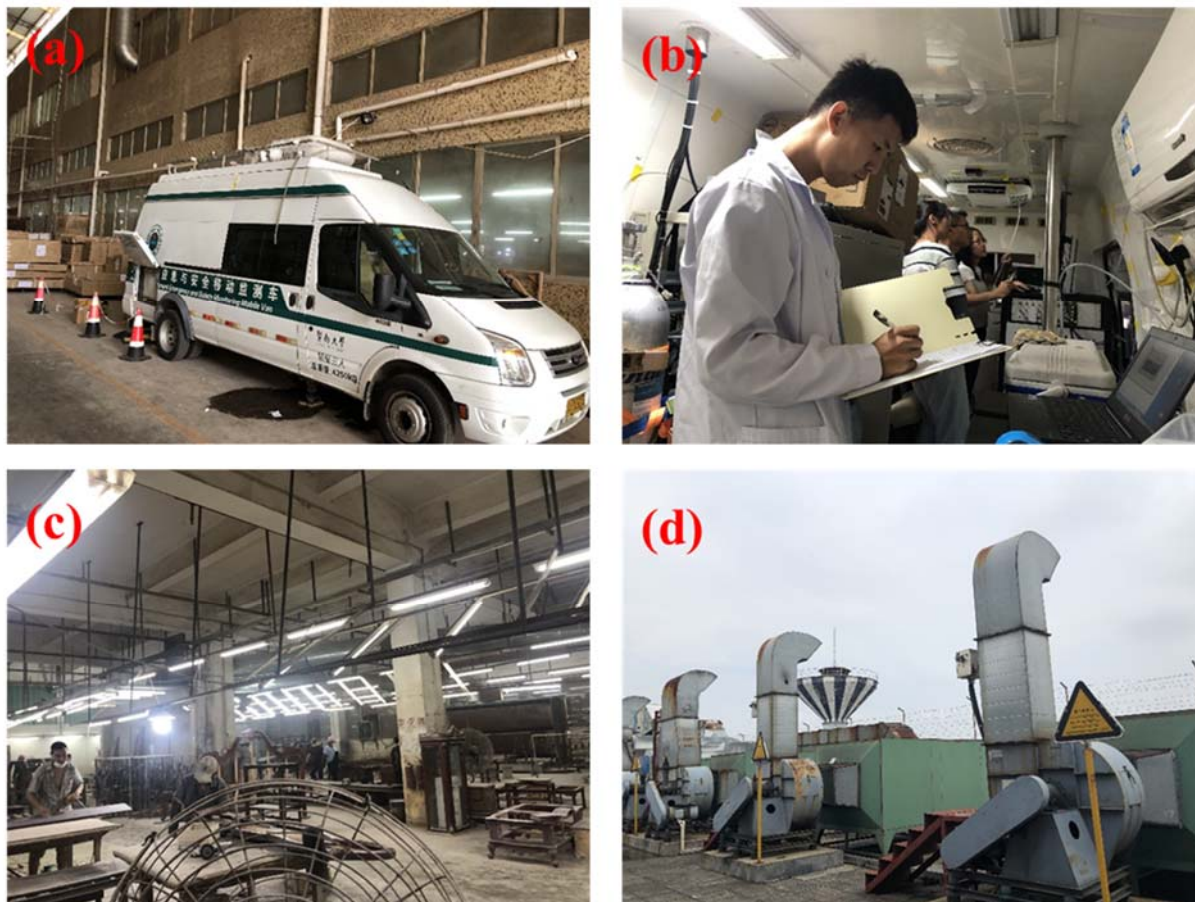
Figure S1. A (a) mobile monitoring vehicle was parking equipped with (b) online measurement instruments at a fixed site which close to (c) the sampling ports of semi-open workshops and (d) stack emissions.
