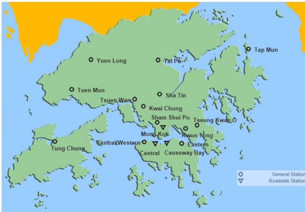
Figure S1. The location of sixteen air quality monitoring stations (AQMSs) in Hong Kong, of which thirteen are general AQMSs including Yuen Long (YL), Tung Chung (TC), Tsuen Wan (TW), Kwai Chung (KC), Sham Shui Po (SSP), Sha Tin (ST), Tai Po (TP), Tap Mun (TM), Tuen Mun (TUM), Tseung Kwan O (TKO), Kwun Tong (KT), Eastern (EN), Central/Western (CW), and three are roadside AQMSs including Mong Kok (MK), Central (CN), and Causeway Bay (CB).
