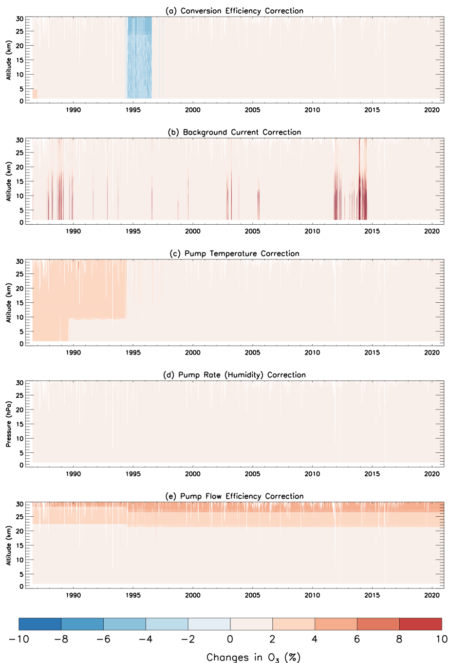
Figure A1. Effect of various corrections on Lauder ozonesonde time series, expressed in percentage changes in ozone.
