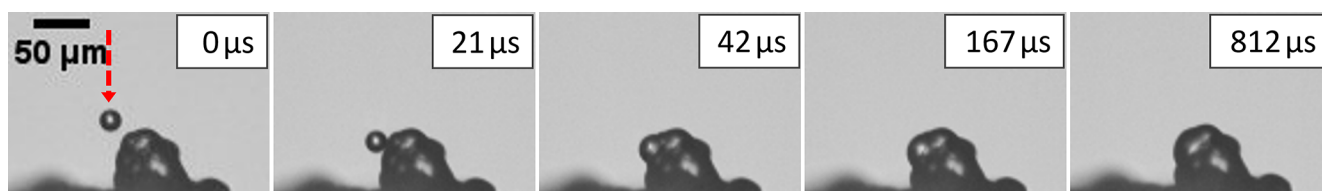
Figure 9. Glancing collision of a droplet of 20\ \mu\text{m} in diameter, resulting in accretion to the rimer surface at -7^\circ\text{C} and 1\ \text{m s}^{-1} . The arrow illustrates the trajectory of the droplet.
