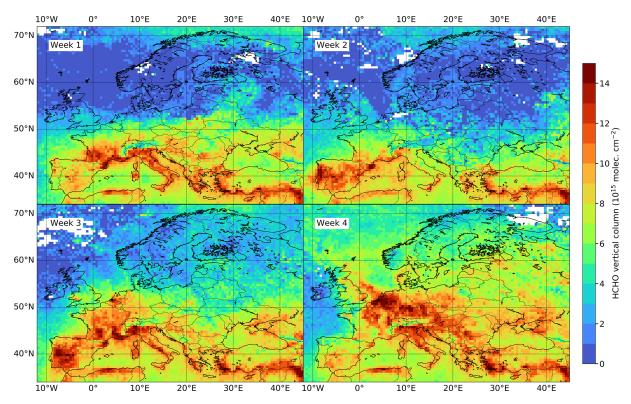
Figure 2. TROPOMI vertical HCHO columns over Europe for the different weeks of July 2019, gridded at  $0.5^{\circ} \times 0.5^{\circ}$ . White regions correspond to grid cells without valid data over the week (usually due to clouds or snow/ice). Week 1 corresponds to days 1 to 8, week 2 corresponds to days 9 to 16, week 3 corresponds to days 17 to 24, and week 4 corresponds to days 25 to 31.
