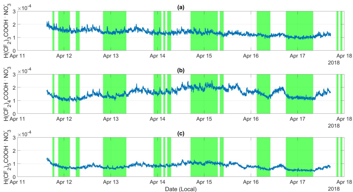
Figure S12 Time series of the fluorinated compounds normalized signal a. \text{H}(\text{CF}_2)_3\text{COOH} \cdot \text{NO}_3^- , b. \text{H}(\text{CF}_2)_4\text{COOH} \cdot \text{NO}_3^- and c. \text{H}(\text{CF}_2)_5\text{COOH} \cdot \text{NO}_3^- . Green patches depict the hours when the Maïdo station is in the FT based on the analysis of the standard deviation of the horizontal wind direction.
