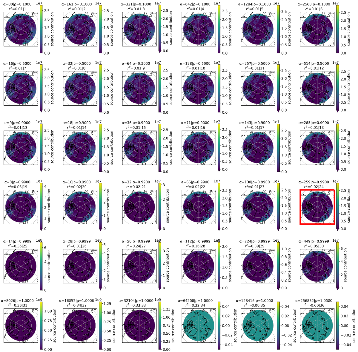
Figure S9. The 36 source region footprint maps of SA produced using the iterative elastic net regularization method in the inverse model. The polygons represent the source region locations identified by the inverse model for various levels of penalization in the elastic net regression method. The elastic net regularization parameters \alpha and \rho , as described in Section 2.6, are included above each map, as well as the correlation coefficient ( r^2 ) and the iteration number. The Iteration 24, outlined in red, was selected in this analysis as it represents known source regions while minimizing noisy regions.
