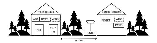
**Figure 1.** Overview of the instruments' measurement locations at the SMEAR II station. Both the main cottage and the aerosol cottage are located inside the forest. The dashed line around WIBS indicates that this instrument measured in both locations and was moved on 3 April from the main cottage to the aerosol cottage. All other instruments stayed at the same sampling location throughout the whole campaign.
